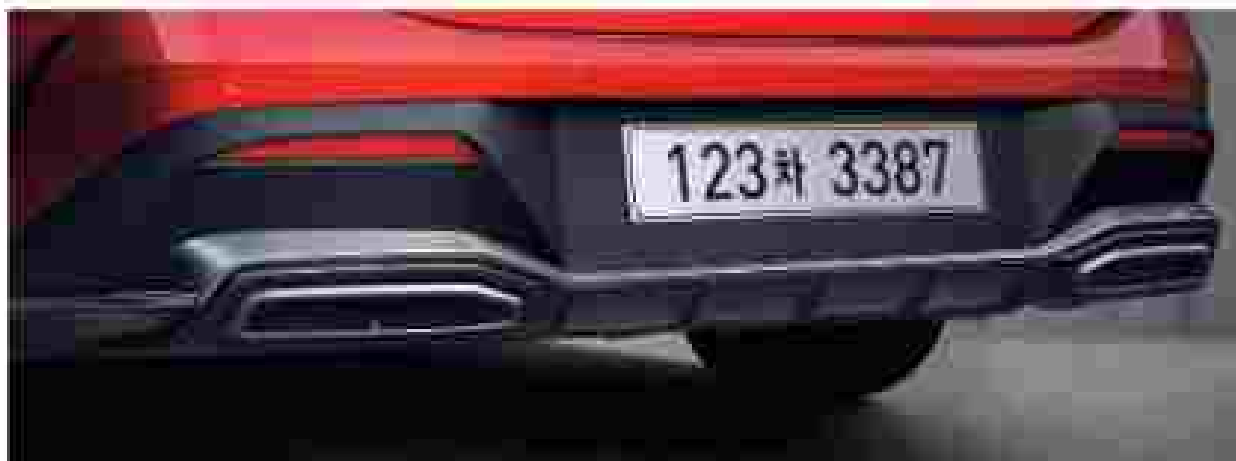
Dual twin tip muffler (2.5T) Dual twin tip muffler garnish (N Line)
